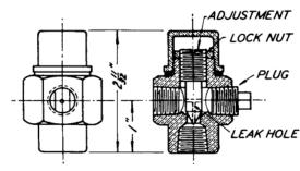
Most types of pressure regulators require a "feeler" pipe for best control. By using this adjustable orifice in the feeler pipe line, rapid pressure fluctuations will be dampened out and more steady control procured.
