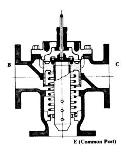
With stem up, B port is open With stem down, C port is open
