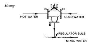
**Figure 1:** Illustrating a simple means for mixing hot and cold water where a rough mixing is suitable.
