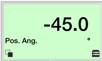
Check the end positions. The angle of rotation is displayed in degrees.
