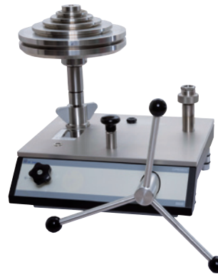
Pressure balance model CPB5800
