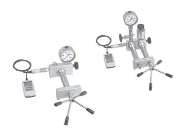
Typical test assembly "hydraulic"
